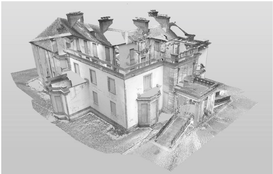
Figure 2.11: Perspective view from laser scan data (Image produced by Dr Marianthi Leon.)
