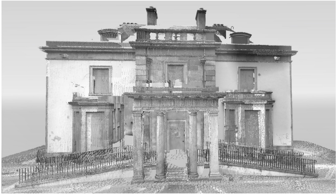
Figure 2.10: Elevation views from laser scan data (Image produced by Dr Marianthi Leon.)
