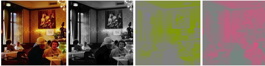
Figure 2.5: YUV colour channels. Image is from (CASIA TIDE) V2.0. Left to right: Image, Y, U, V, (best viewed in colour)
