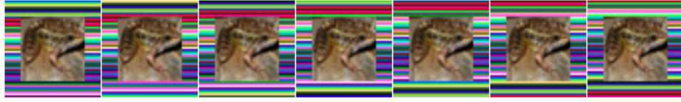
Figure 4.5: The 7 frames of a short, synthesised video. The invariant image is overlaid onto a moving background of upwards scrolling horizontal lines. The background border adds 8 pixels on each side so that of the 9 macroblocks comprising the image, 8 contain moving data. This forces the compression codec to use predicted blocks with motion compensation, rather than skipped blocks as it would with a repeated image.
