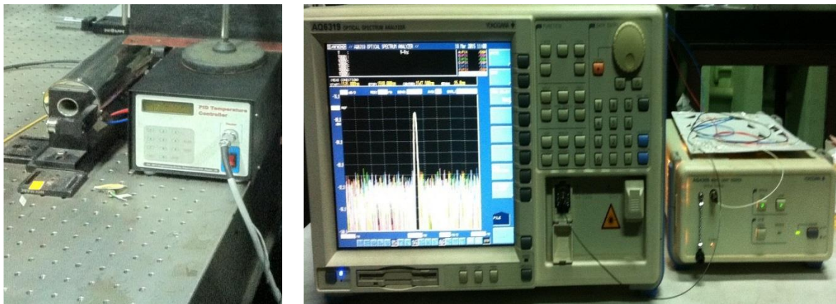
Figure 4.14: Experimental set up used for FBG temperature analysis for temperatures above 100 °C
