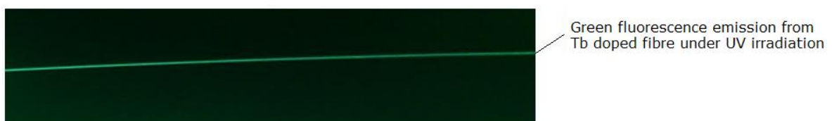
Figure 5.40: Green photoluminescence emission from Tb doped fibre when irradiated using UV LED in a dark room
