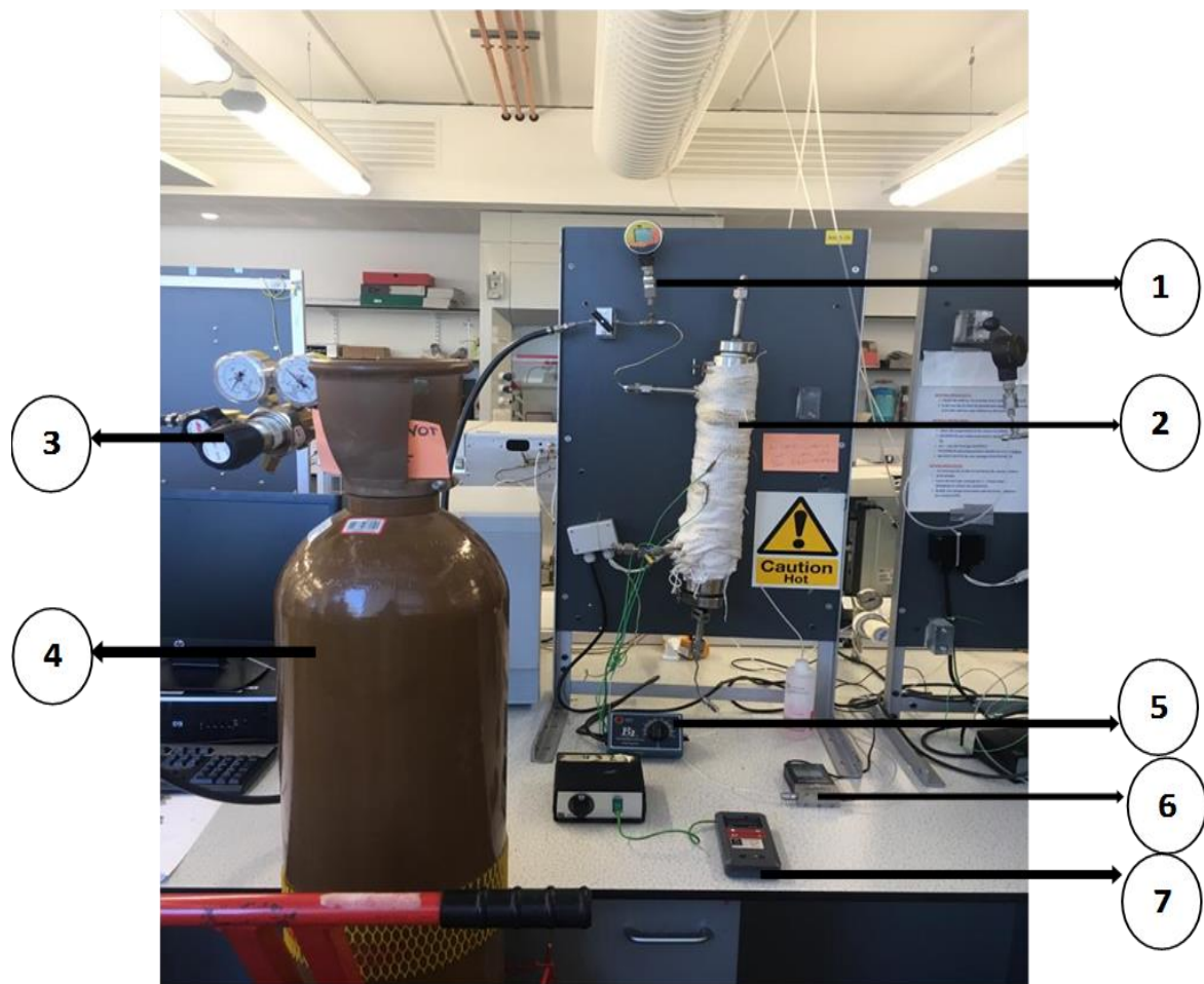
Figure 3 Experimental set-up showing all equipment including; pressure gauge(1), membrane module covered with heating tape(2), gas regulator(3), gas cylinder(4), heat regulator(5), volumetric meter(6) and temperature indicator(7)
