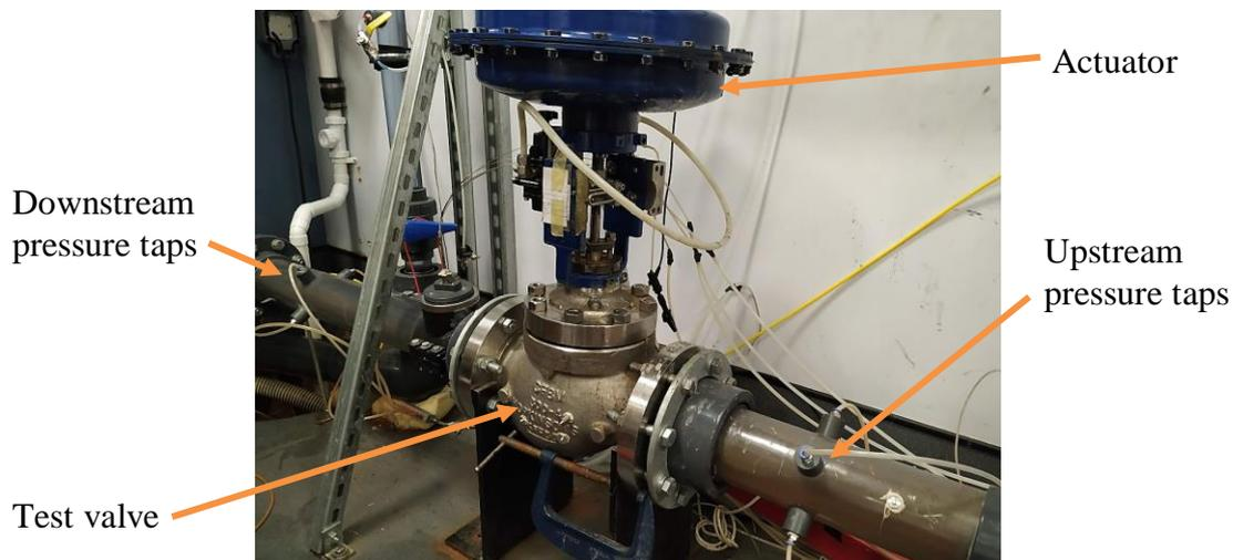
**Fig. 4.** Test valve set-up
