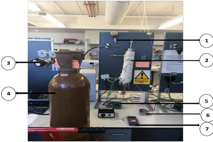
Figure 1 Experimental set-up showing all equipment including; pressure gauge(1), membrane module covered with heating tape(2), gas regulator(3), gas cylinder(4), heat regulator(5), volumetric meter(6) and temperature indicator(7)
