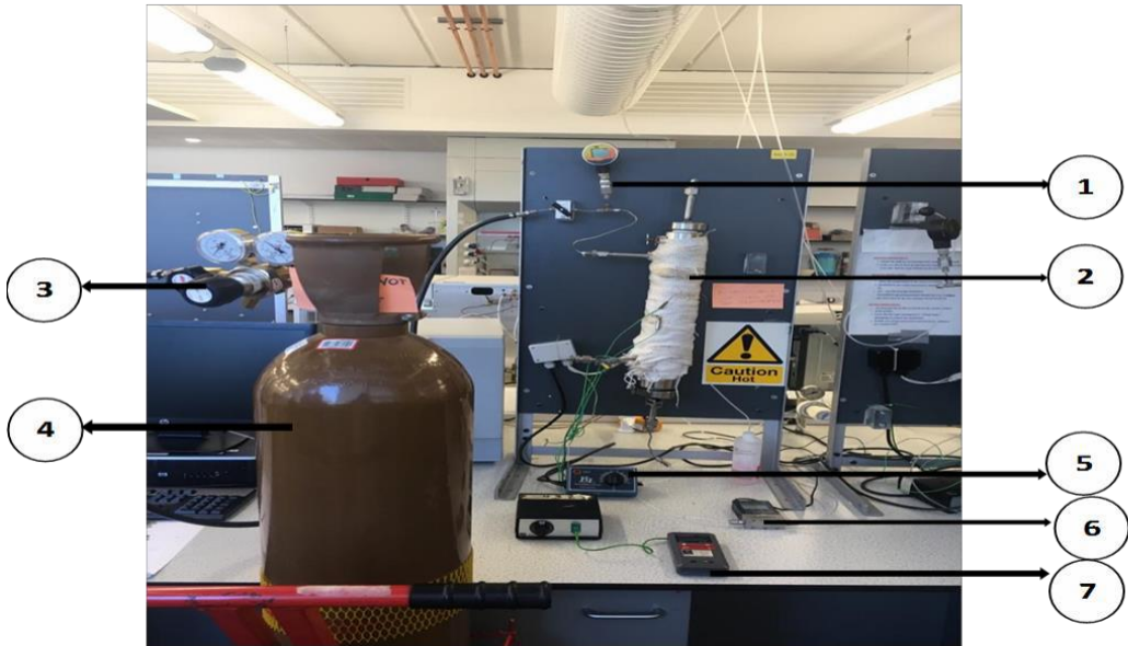
Figure 1 Experimental set-up showing all equipment including; pressure gauge(1), membrane module covered with heating tape(2), gas regulator(3), gas cylinder(4), heat regulator(5), volumetric meter(6) and temperature indicator(7)
