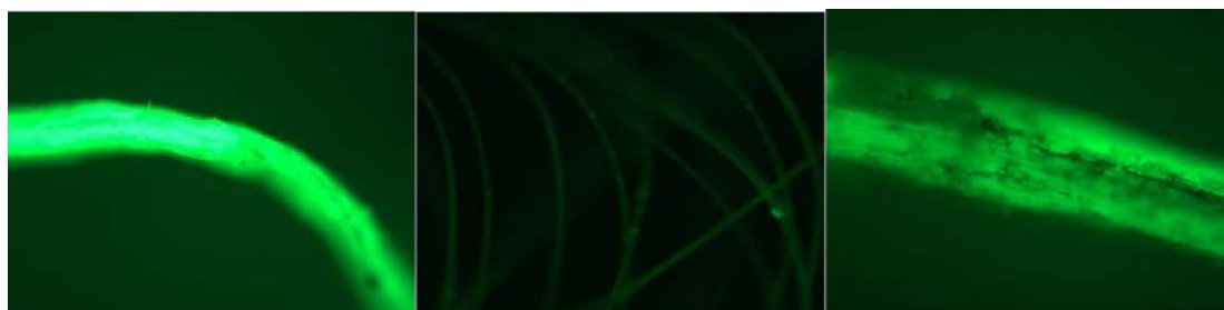
Figure 7: Fluorescence of (a) barley root, (b) acrylic and (c) coconut fiber upon Nile Red staining
