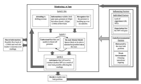
Fig. 2. Possible driller's SA for the first Negative Pressure Test at 5pm.
