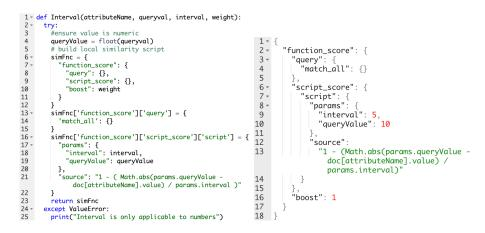
**Fig. 3.** Python severless function for gener-**Fig. 4.** Generated Painless script for Inating Interval local similarity script terval local similarity
