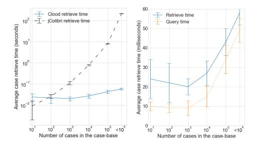
Fig. 8. Case retrieve times as casebase size increases. Both axes are log scales.
