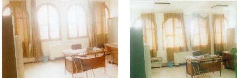
Figure 6a : views revealing the difference, at the window vertical plane and the overall space, between an uncontrolled and a controlled (by means of curtains) luminous ambience in an office of Biskra. (2 photos on top)
