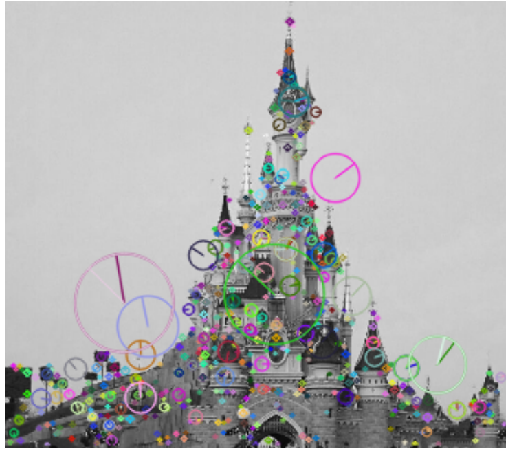
Figure 2.1: SIFT key proposals drawn across the image by applying the SIFT algorithm. The center of the circles represents the key points and the circle is the neighbourhood considered.
