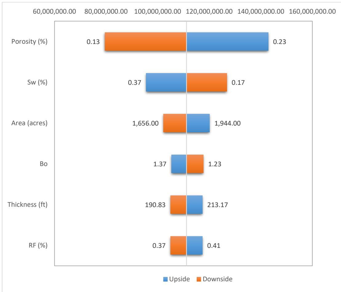
**Figure 2. 16 Showing porosity and water saturation as the most sensitive for reserve estimation with both P10 and P90 cases for Ness Reservoir, Don Field, North Sea.**
