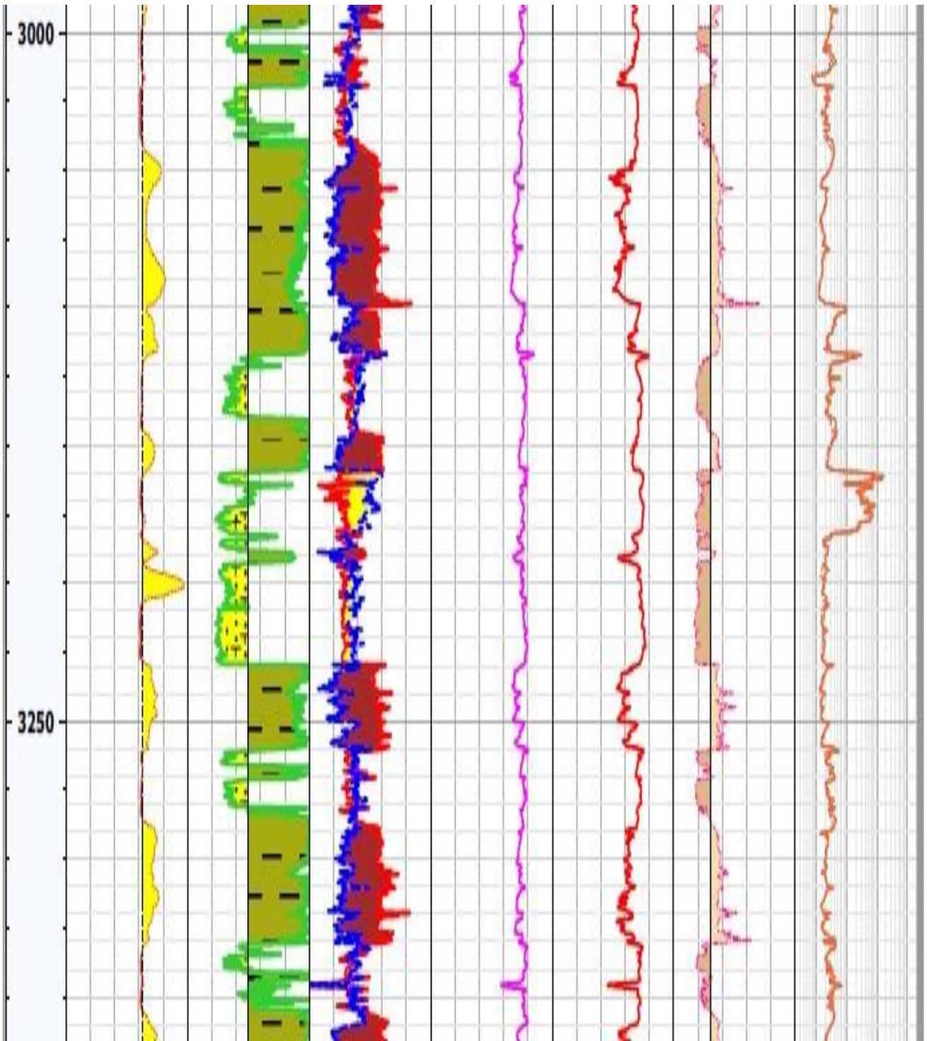
Well log showing Shallow reservoir from which mechanical properties were evaluated
