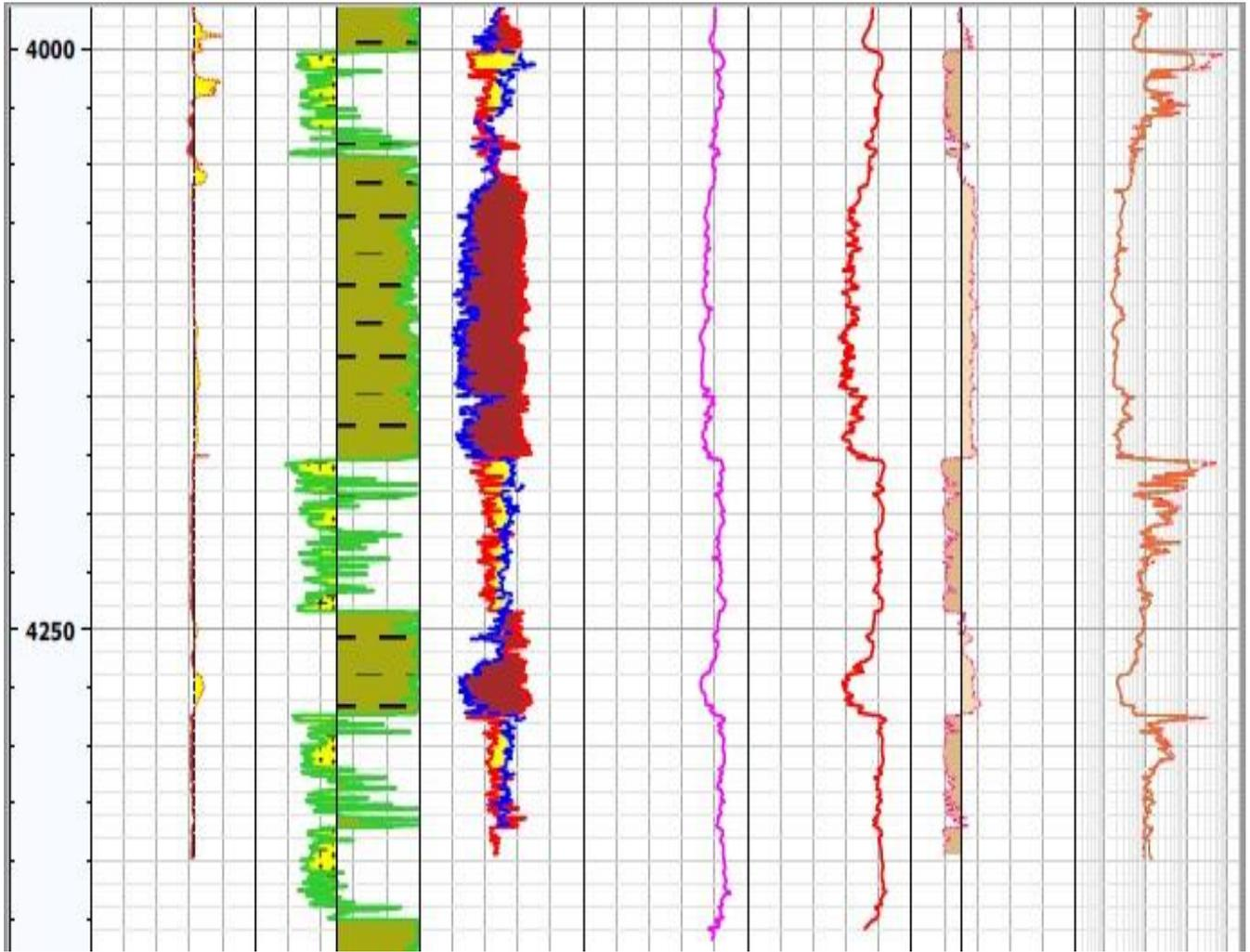
Well log showing Deep reservoir from which mechanical properties were evaluated.
