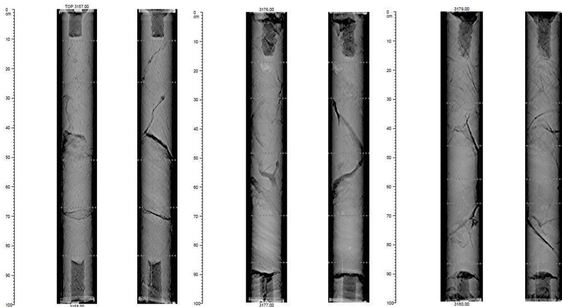
**Figure 4.7.** X-ray computerized tomography scan of core showing cracks (or induce fractures) for Wabi 05 well.
