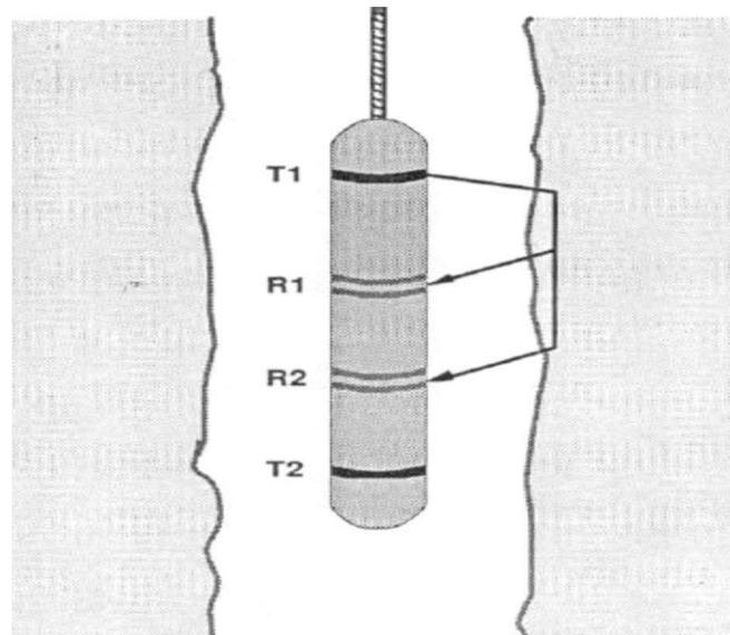
**Figure 3.2.** The Sonic Logging Tool. (Martey, 2000).
