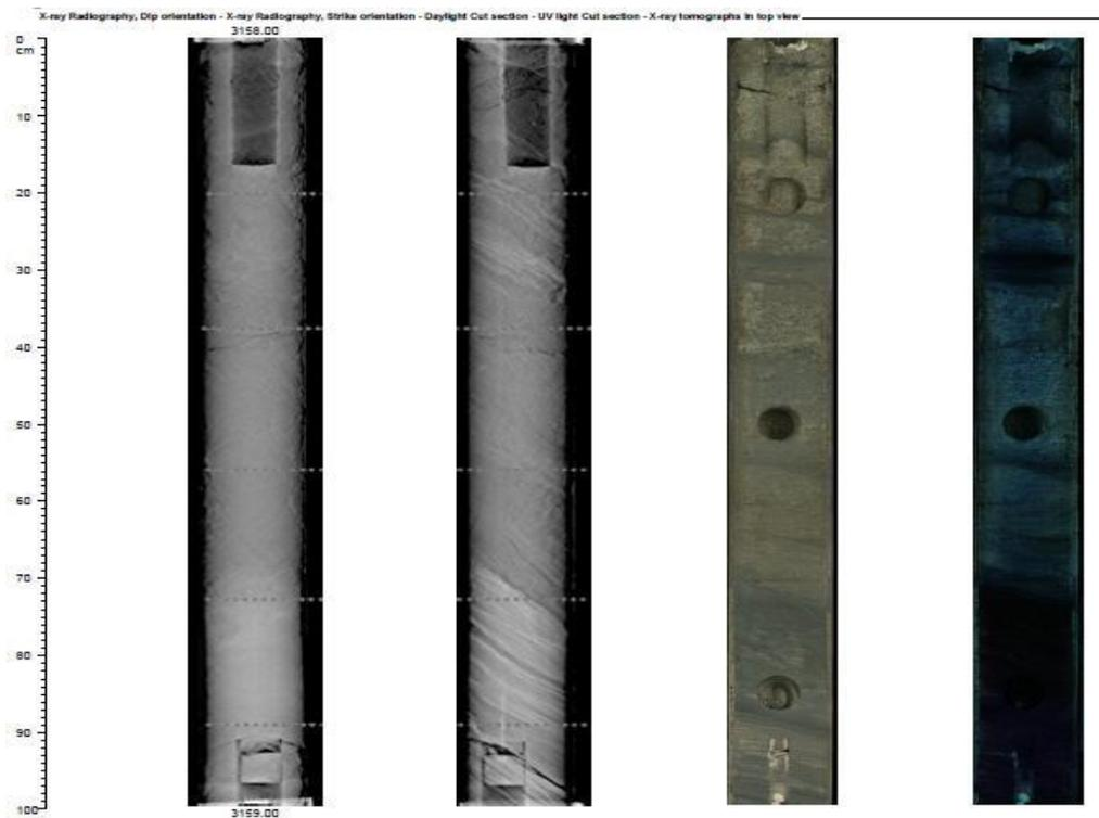
1&2): X-ray radiography showing dip and strike orientations,3.)Daylight cut and 4.) UV light cut section
