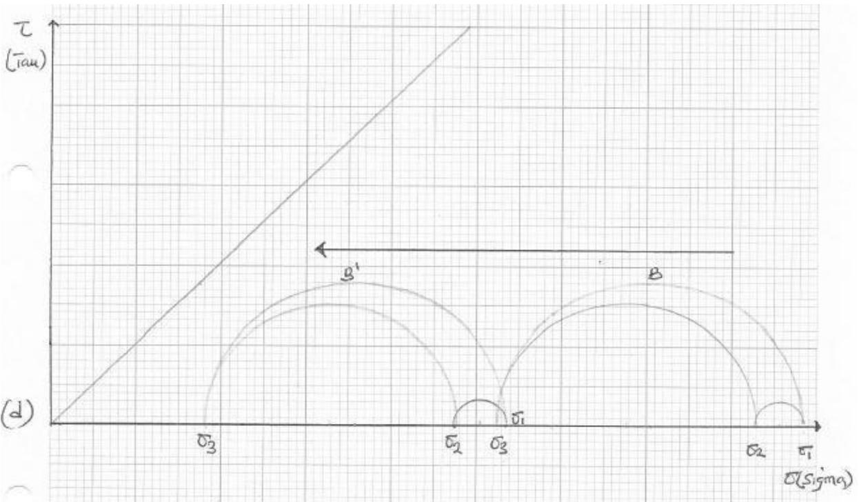
3D Mohr diagram construction for Wabi 05 showing movement of Mohr circle for injectivity scenarios
