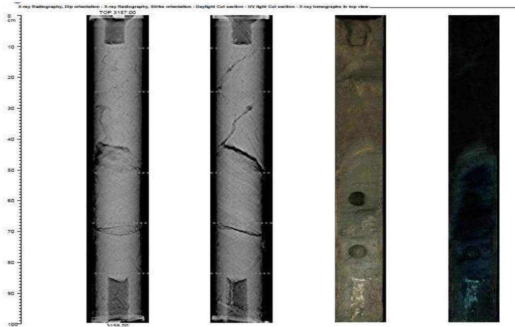
1&2): X-ray radiography showing dip and strike orientations,3.)Daylight cut and 4.) UV light cut section
