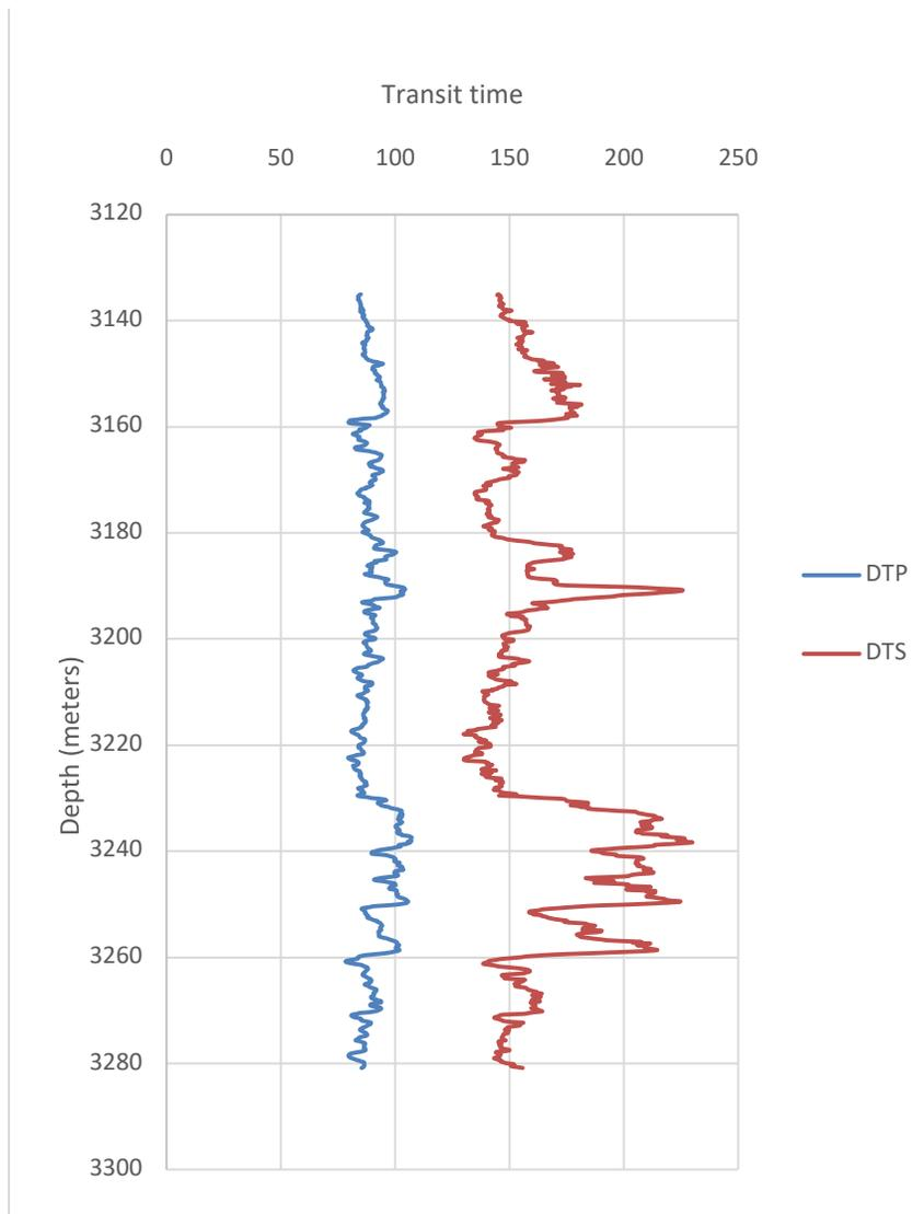
**Figure 4.2.** Slowness ( $D_{TP}$  and  $D_{TS}$ ) profile for Wabi 5A reservoir. Where  $D_{TP}$  is the P-wave travel time and  $D_{TS}$  is the S-wave travel time
