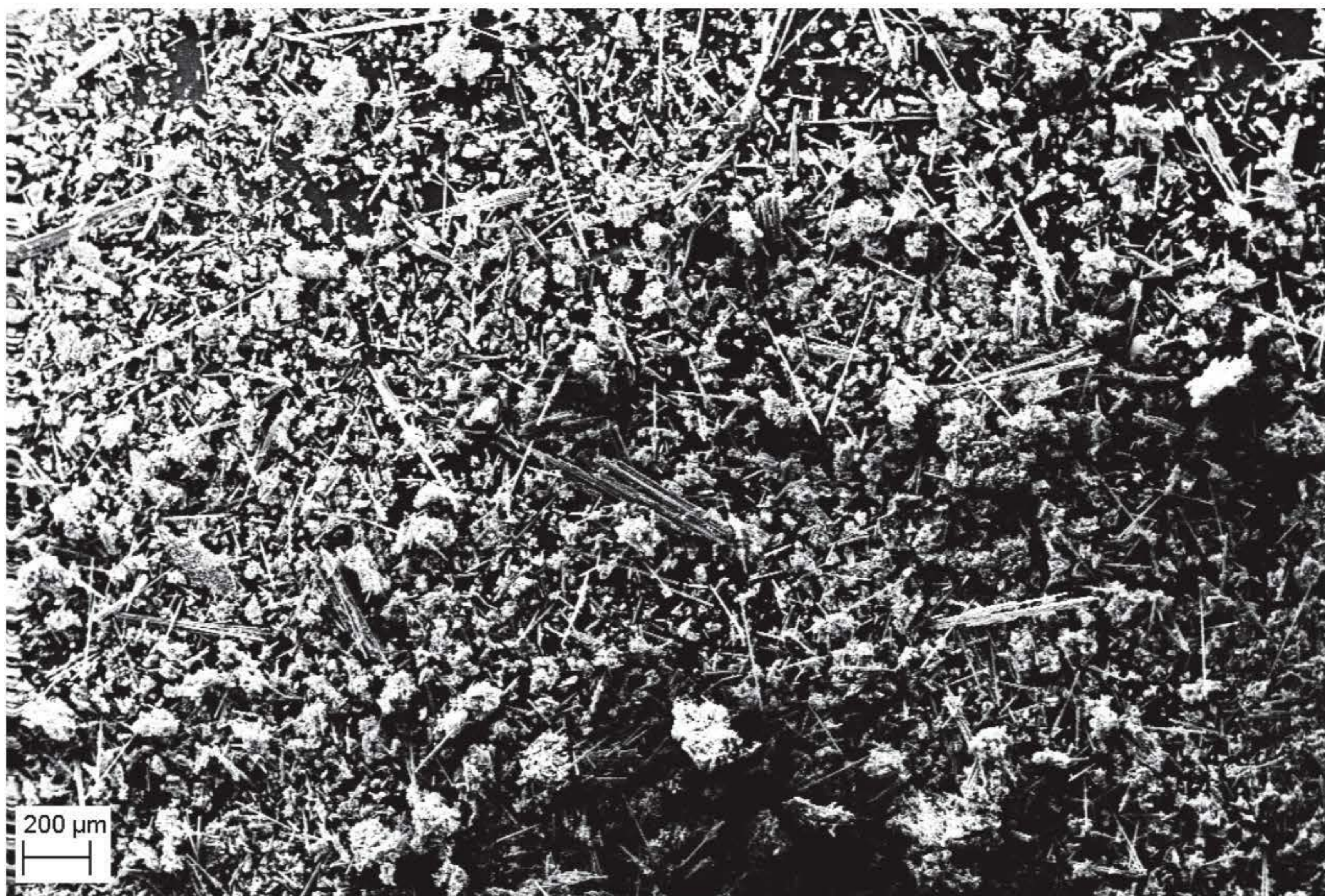
Figure 110: Deposited particles collected in sampling tray placed directly below drilling from EP/CF/GO 0.5 wt. % sample.
