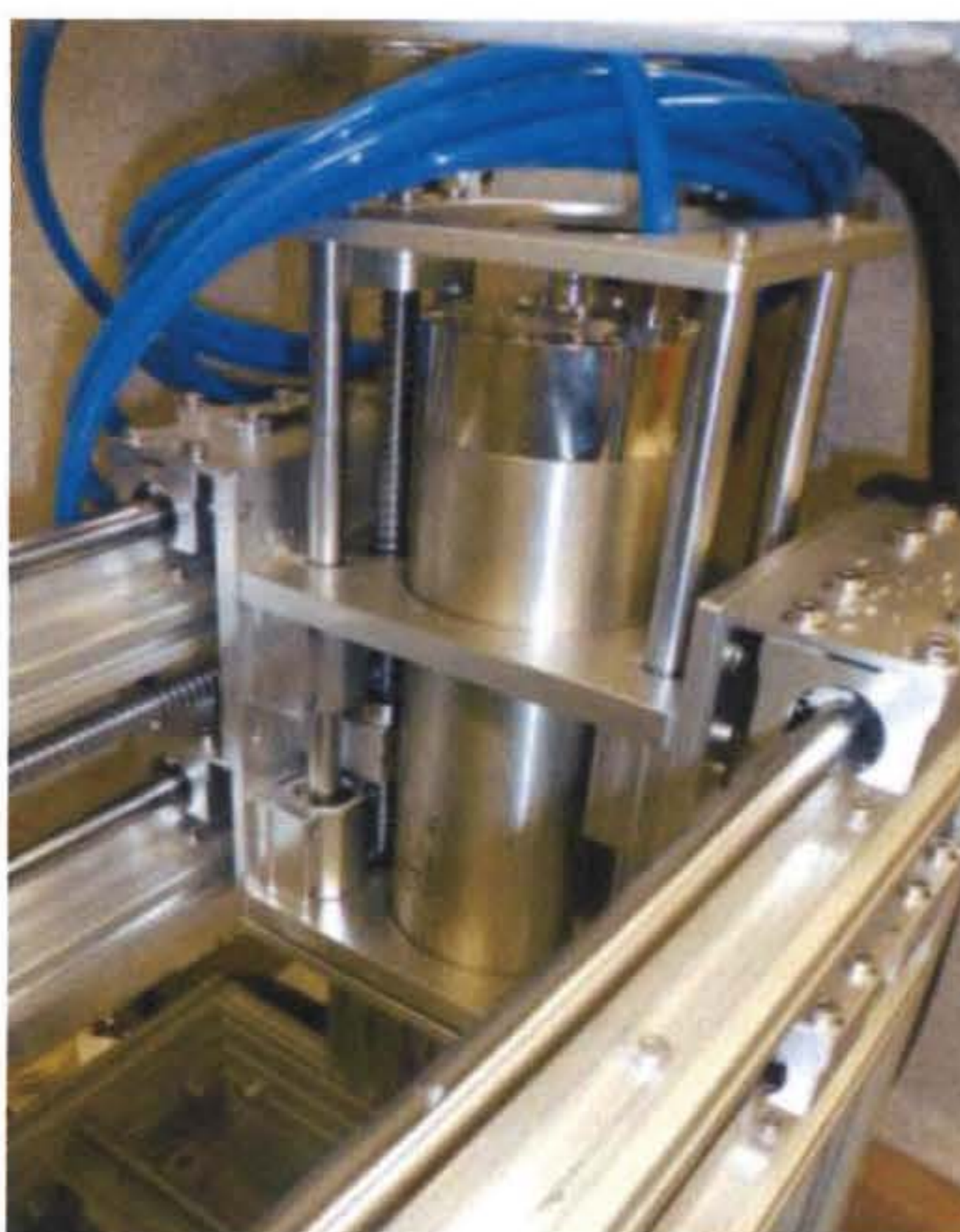
Figure 7: Water cooled and sealed spindle drill system implemented in the prototype developed within SIRENA
