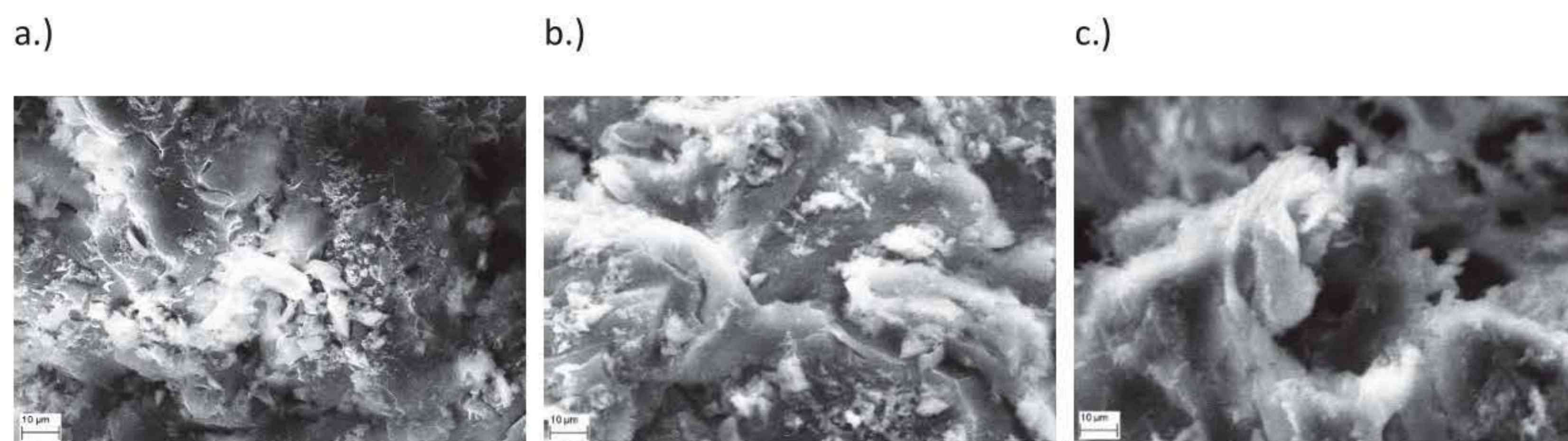
Figure 99: SEM images of collected debris from sampling tray within chamber of a.) Neat Epoxy b.) EP/CNF and c.) EP/CNT samples.
