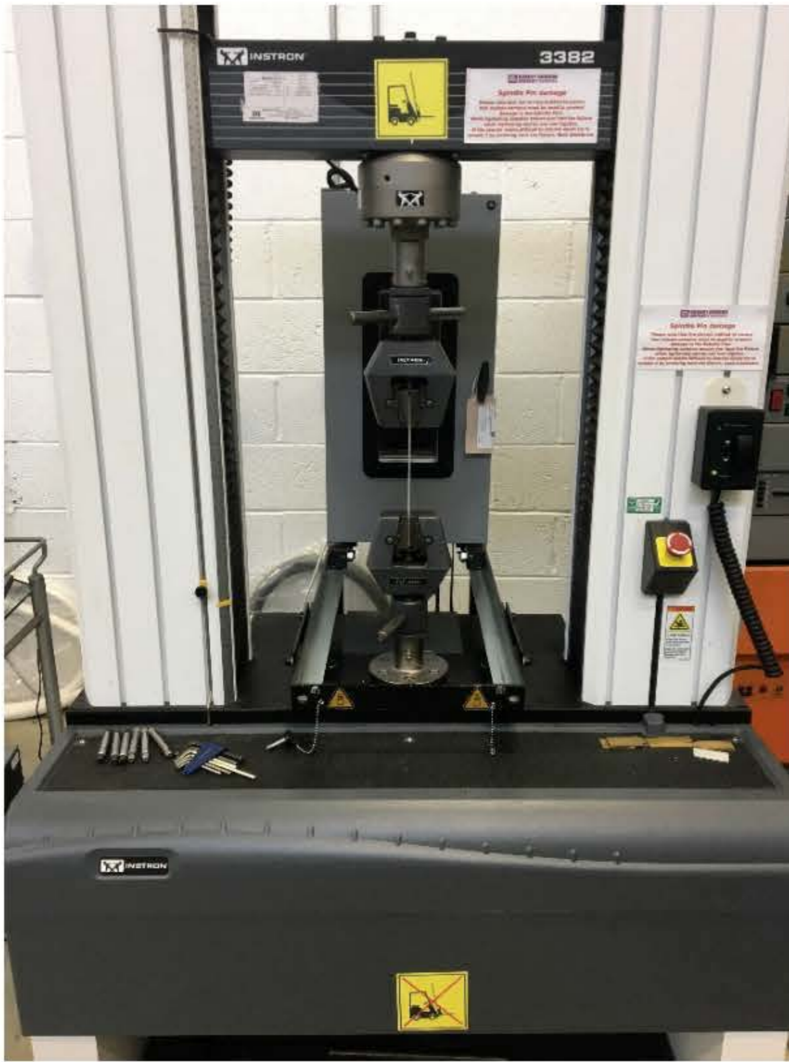
Figure 17: Instron 3382 universal testing system used for a.) tensile test (ASTM D3039, 2017) and b.) 3-point flexural test (ASTM D7264M, 2015).
