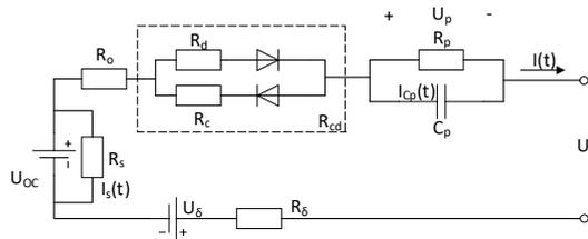
**Figure 4.** The improved equivalent model of IECM
