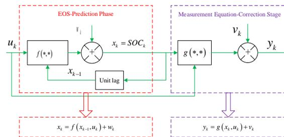
Figure 6. SOC estimation model framework for power LIB
