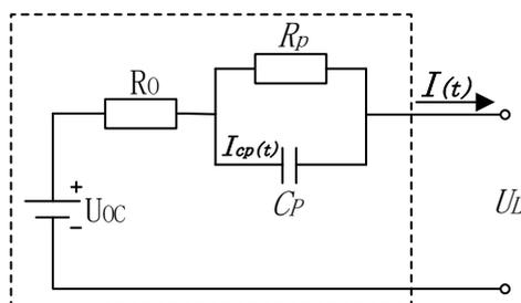
Figure 2. Thevenin equivalent diagram
