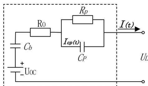
**Figure 3.** PNGV model diagram
