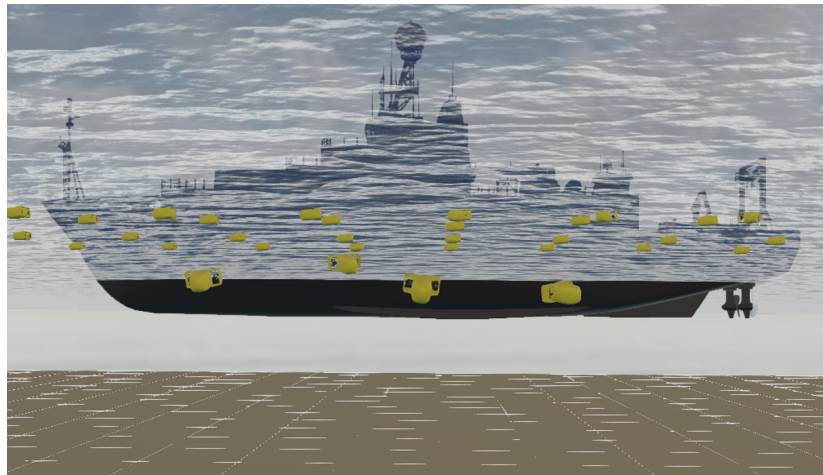
Figure 7. Underwater Webots simulation scene of 50 AUVs deployment, the USBL transceiver is hull-mounted on the deployment vessel.
