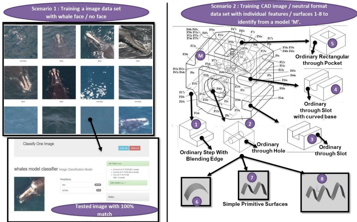
Fig. 6. Schematic representation of identified whale face from an image data set alongside image / CAD data set consisting of manufacturing features / surfaces.
