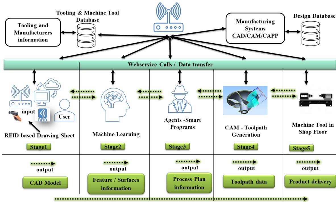
Fig. 1. Five Stage IoT based Industry 4.0 Architecture for Integration of Design and Manufacturing Systems
