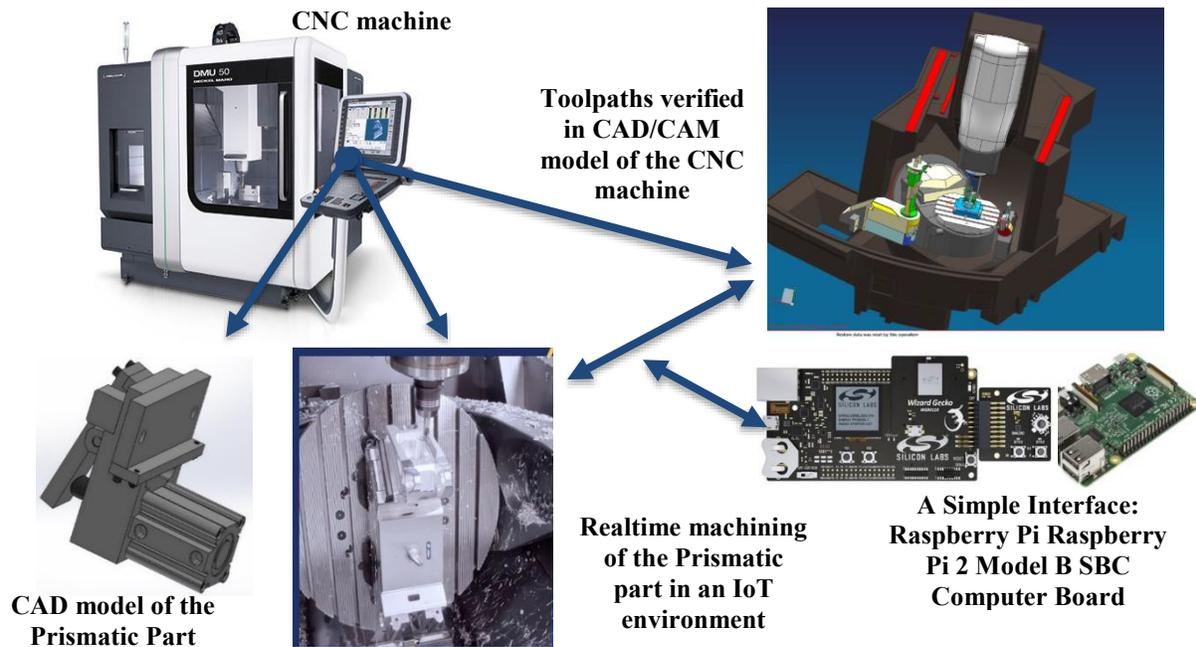
Fig.8. CAD/CAM to machine transfer for real time manufacturing
