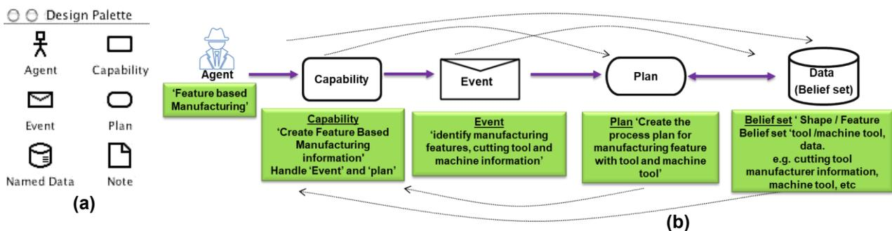
Fig.7. A simple Agent for 'Feature based Manufacturing' based on BDI concept
