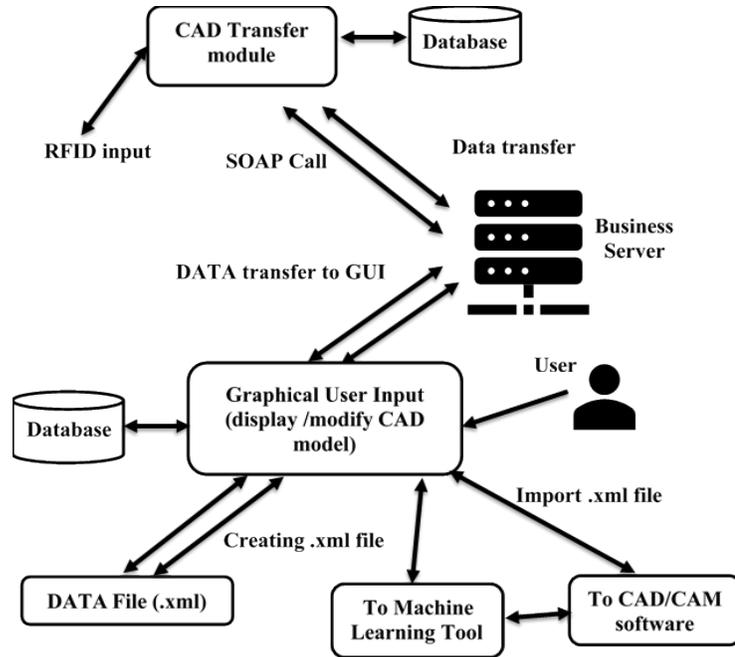
Fig. 5. Business model of GUI prototype with SOAP based protocol for CAD model retrieval.
