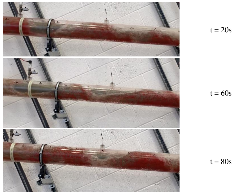
595 Fig. 9. Particle transport dynamics with time in the slug flow pattern
