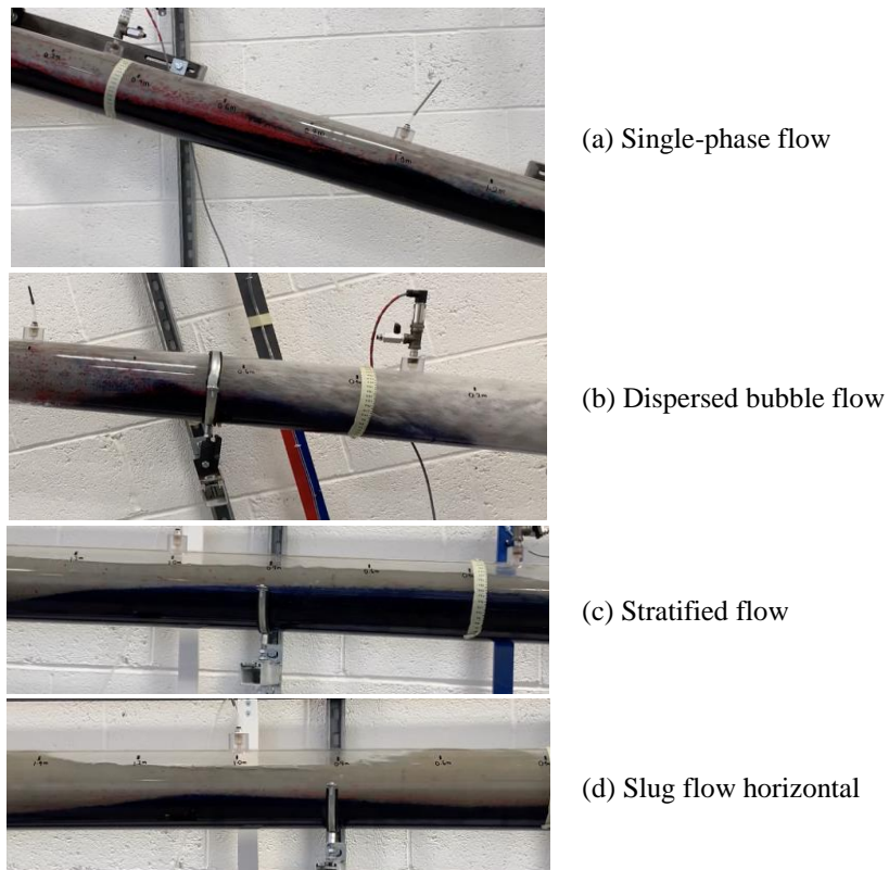
938 Fig.A.2: Examples of different cutting transport mechanisms existing in the different gas-liquid flow patterns 939
