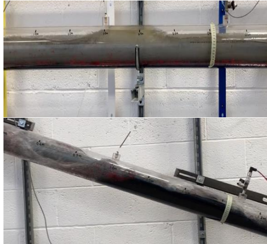
Fig.A.5: Comparison of particle transport in the horizontal and inclined annuli for water and air (top) moving bed with slug flow pattern in the horizontal annulus and (bottom) stationary bed for the slug flow pattern in 30° inclined annulus
