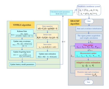
Figure 2. The process of estimation of SOC by the VFFRLS-SRAUKF algorithm
