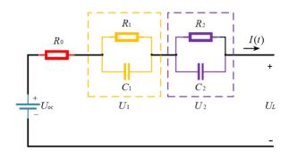
Figure 1. Second-order RC equivalent circuit model
