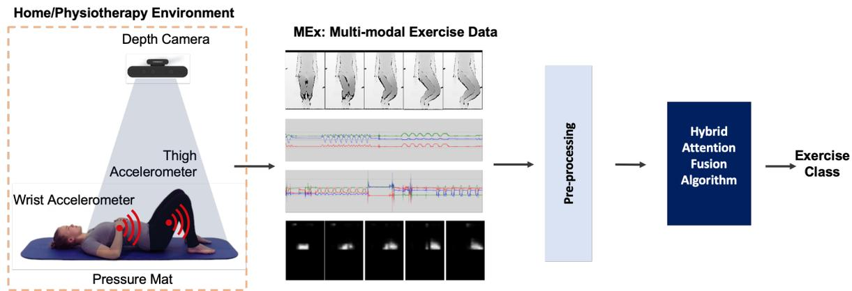
Fig. 2. Exercise recognition with heterogeneous multi-modal sensors
