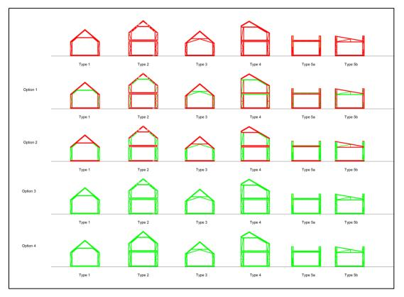
Figure 13. Truss options. Red = milled timber; Green = whole timber.
