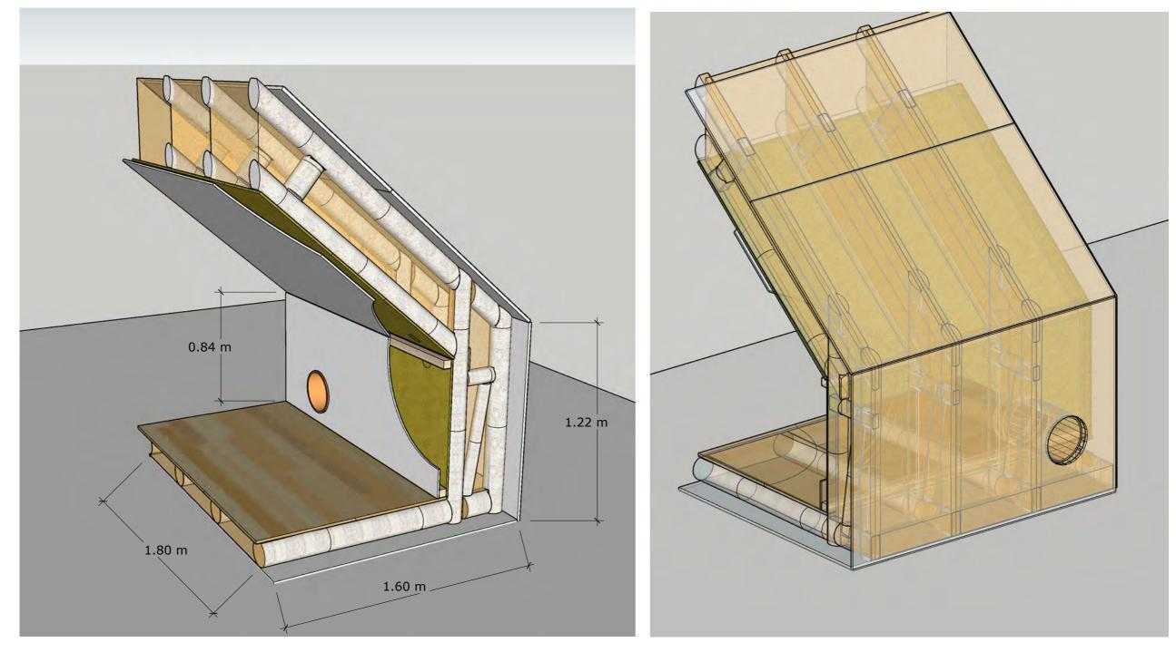
The figures above show two views of a truss demo module. The exact trusses used in this design are yet to be determined, these figures are for illustration and approximate size only.
