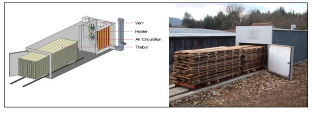
Figure 25. Kiln drying.
