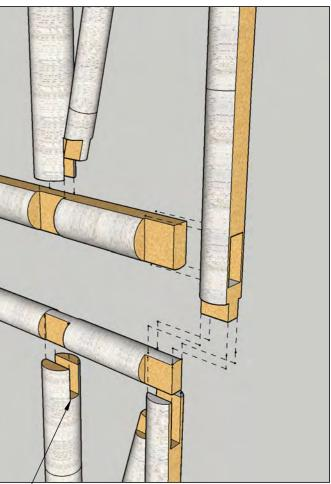
Universal tenon size Can be used for main timber junctions. smaller tenons for minor connections
