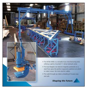
Figure 29. Truss press.
