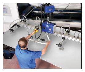
Figure 20. Suction cup lifting equipment.
