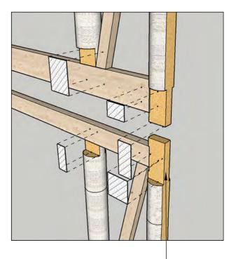
Whole timber thickness reduced to same thickness as milled timber (47mm shown)•–
