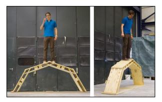
Figure 5. Double-layer arch.
