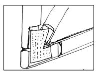
Figure 10. Gang-nail plate connection.
