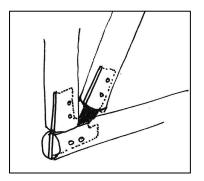
Figure 9. Flitch plate connection.
