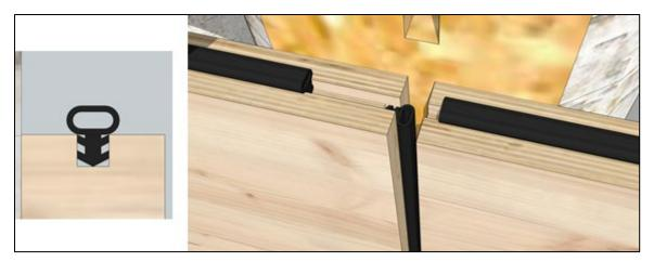
Figure 15. Dry Elastomer seals.
