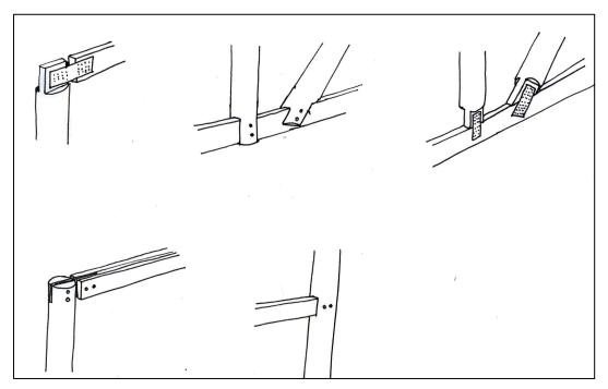
Figure 12. Hybrid connections.
