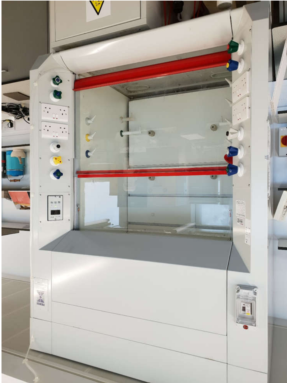
Figure 6-16 Fume cupboard for exhausting gas.
