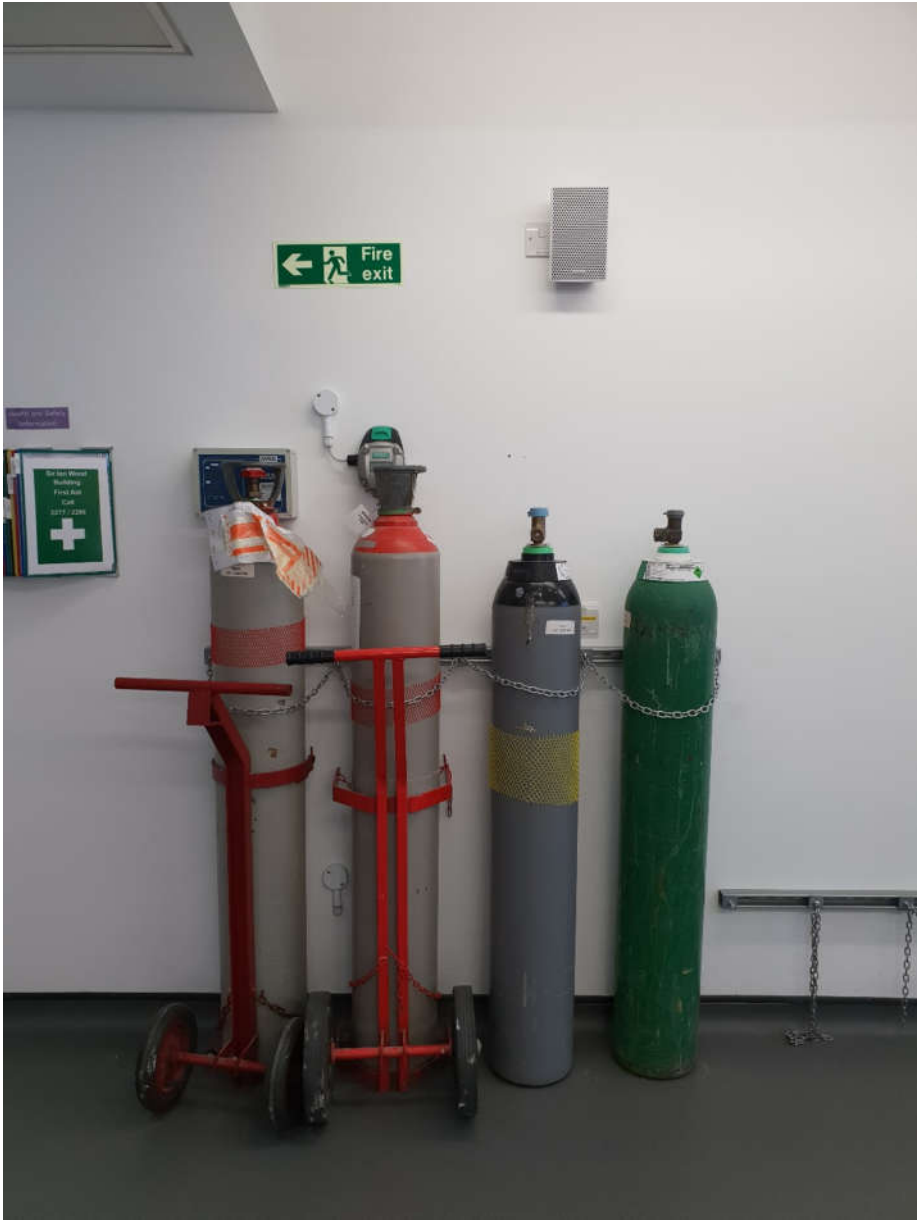
Figure 6-15 Gas cylinder for storing EOR gases at 250Bar ordered from BOC, UK.
