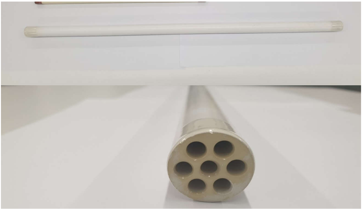
Figure 6-8 Areal and Cross-Sectional view of 15nm and 2.56cm outer diameter core sample.
