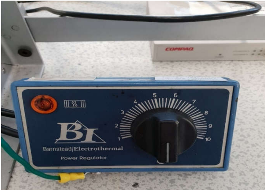
Figure 6-17 Barnstead Electrothermal Heat regulator the heat generated by the heating element wrapped around the core holder.
