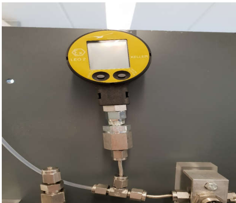
Figure 6-12 Keller Pressure gauge for controlling and monitory of pressure flow in the core.
