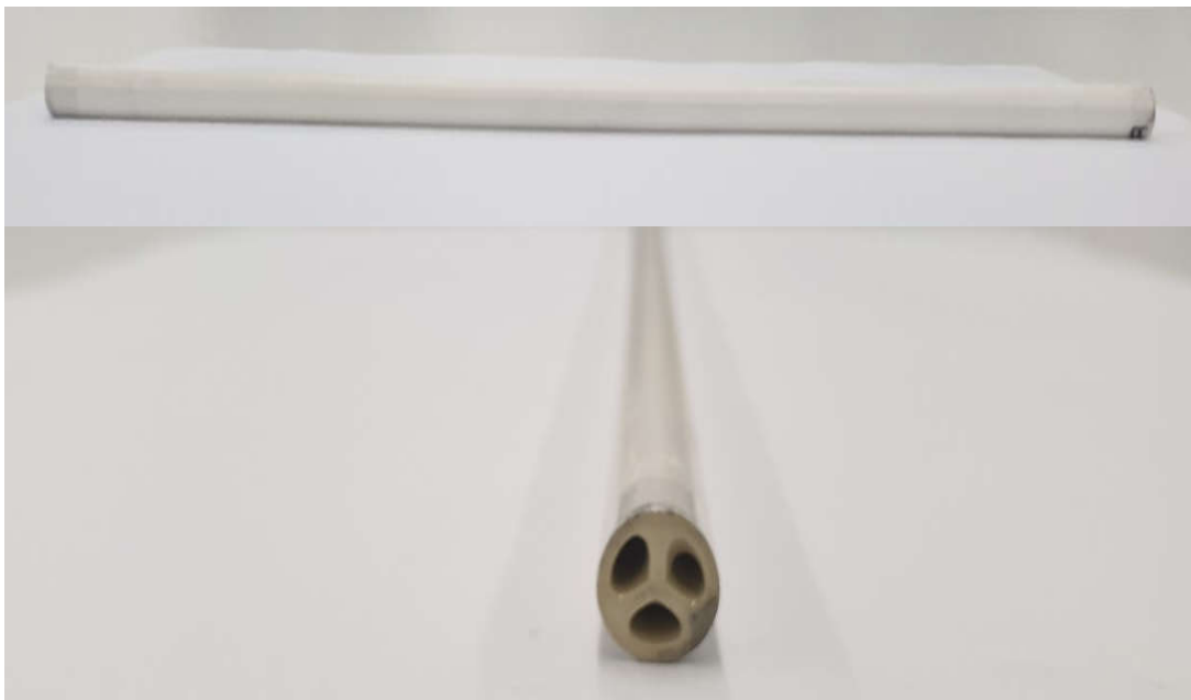
Figure 6-6 Areal and Cross-Sectional view of 6000nm and 1.02cm outer diameter core sample.
