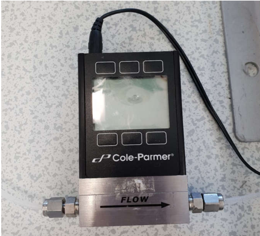
Figure 6-13 Cole-Parmer flowmeter for taking flow rate at steady state (x2).
