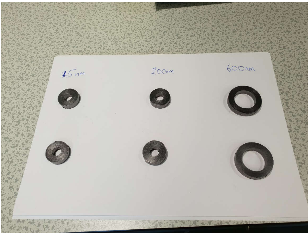
Figure 6-14 3 sizes of granite seal to seal off the core and core holder from gas leaks.
