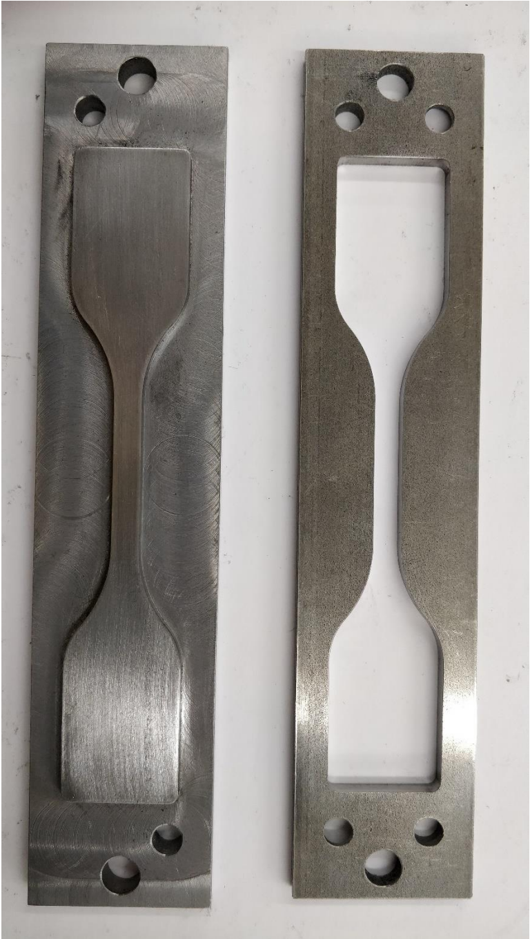
Figure E.5. Upper and middle portions of the metal die fabricated for composite dog bone sample preparations.
