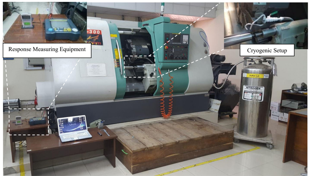
Fig. 2 Cryogenic experimental setup (a) CNC turning center with response measuring equipment and cryogenic setup (b) dual nozzle configuration (c) cryogenic cylinder schematic diagram
