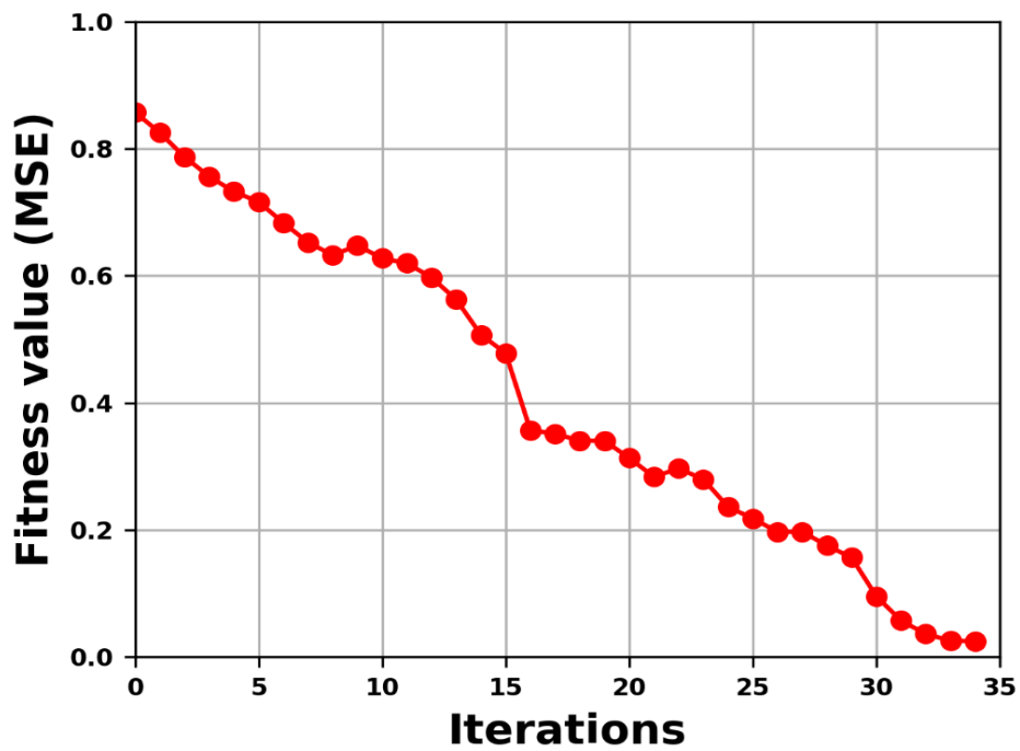
Figure 6-8: Convergence profiles of the constructed surrogate model (PSOASM) for multiphase pipeline leak detection.
