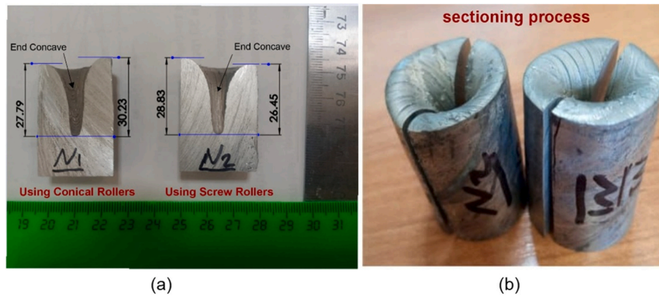
Fig. 13. End-tightening depth variation in A2024 bars during RSR with different roller profiles: (a) Sample sectioning with groove dimension, (b) General view of the sectioning process.
