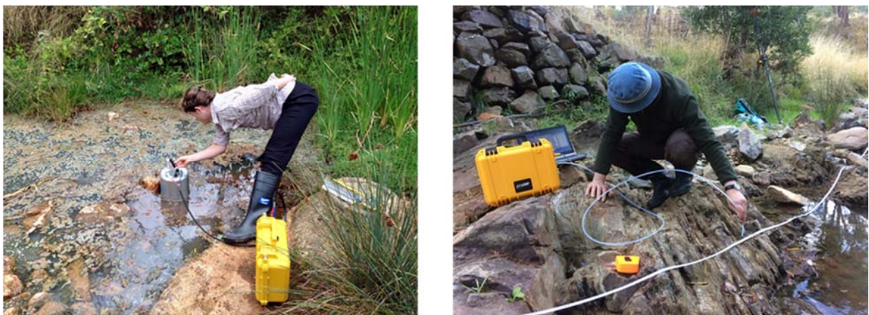
Figure 1 Measuring CO 2 seepage at sites in Daylesford, Vic. Images from Jen Roberts (L) and Andrew Feitz (R).
