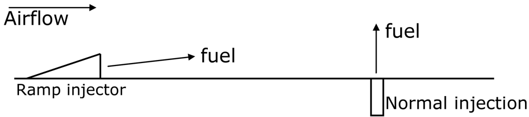
Fig. 2 Normal and ramp injection.
