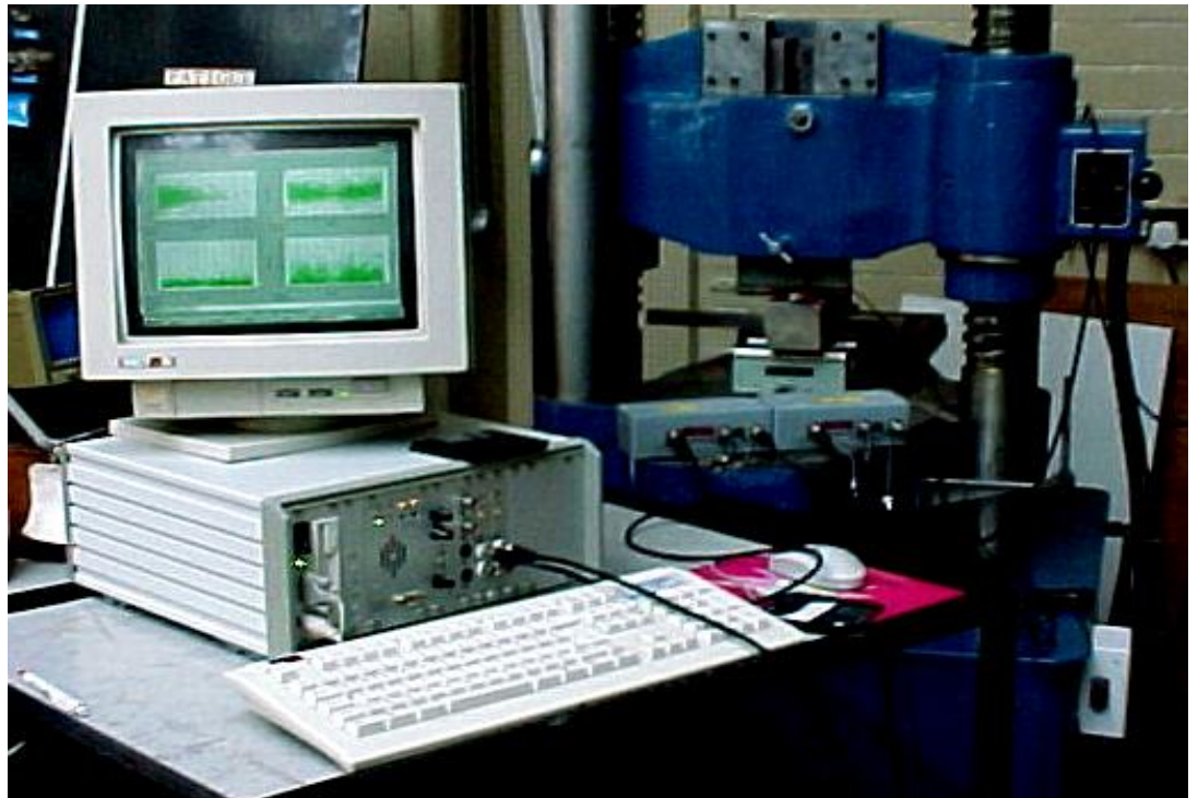
Figure 4.6: The Acoustic Emission (AET) AMSY4 AE Vallen System
