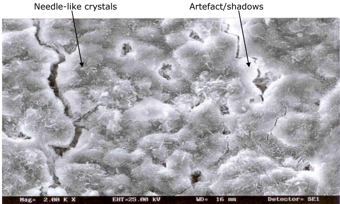
Figure 5.15: Microscopic Structure of Mortar Sample with Sodium Sulphate, 2000 times magnification
