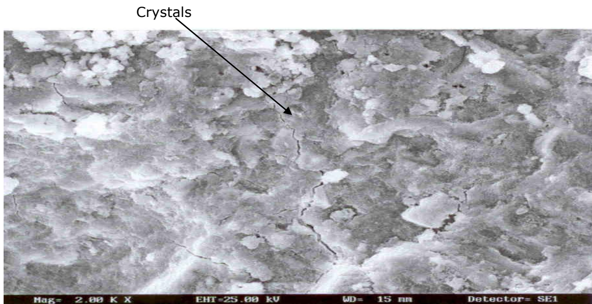
Figure 5.21: Microscopic Structure of Mortar Sample with Calcium chloride-2000 times magnification
