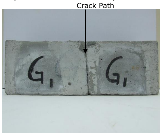
Fractured Sample g) Plain Mortar
