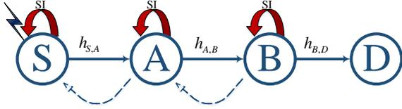
Fig. 1: Example of a route  $R = \{S, A, B, D\}$ . Straight lines represent the intended transmission, while dotted lines represent neighbouring interference, and the red semi-circled arrows represent SI.
