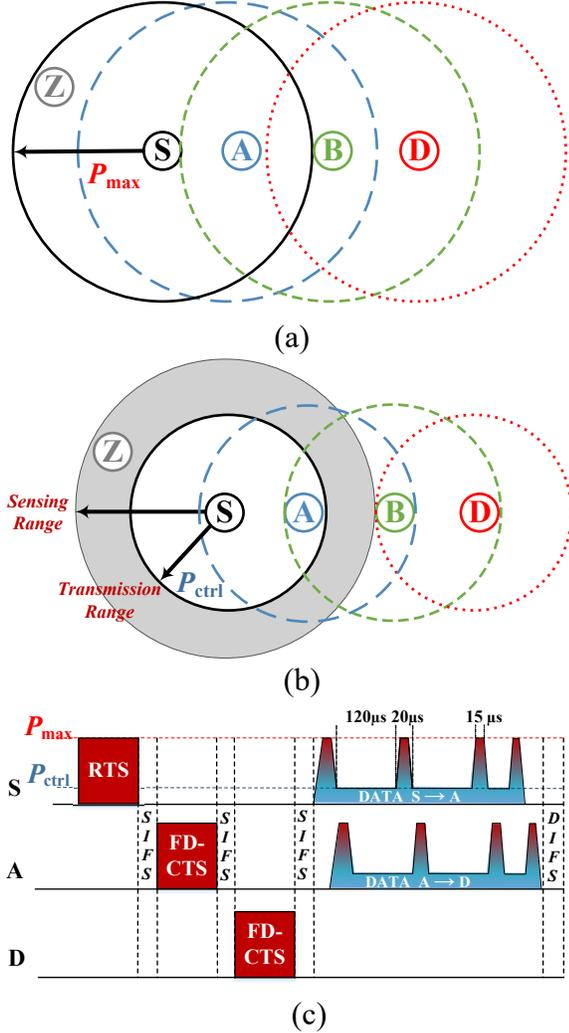
Fig. 2: (a) Ranges of nodes transmitting control signals using  $P_{max}$ ; (b) ranges of nodes after application of power control; (c) illustration of a uni-directional FD transmission at the MAC layer.
