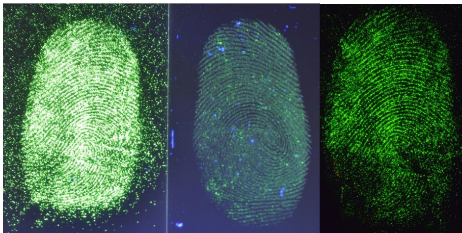
Figure 10: Comparison of fingerprints developed with \text{Na}_3[\text{Tb}(\text{DPA})_3] \cdot 9\text{H}_2\text{O} (left side) and batch 2 (middle) excited with UV light of 254 nm. The picture on the right shows the fingerprint developed with \text{Na}_3[\text{Tb}(\text{DPA})_3] \cdot 9\text{H}_2\text{O} and the use of filters to reduce background fluorescence.
