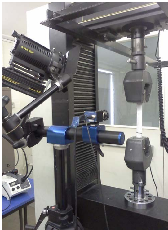
Figure 3. DIC technique applied to provide micro-scale information.
