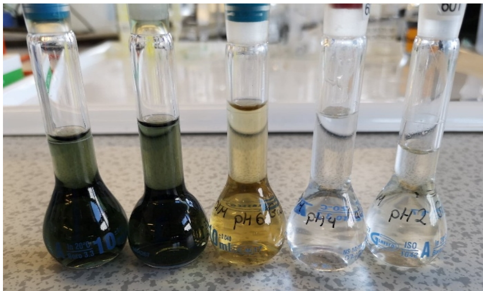
Fig. S6. Images of Gallic acid solutions at different pH, showing a very dark solution at a pH 10, that becomes brighter as the pH reduces to pH 8 to pH 2.
